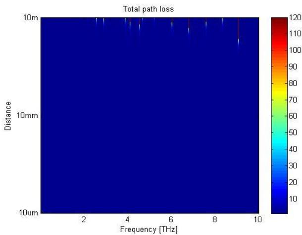
Figure 8. Path loss in water molecule -0.001%
