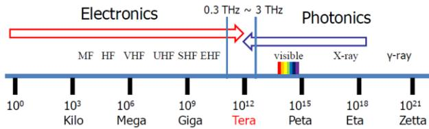
Figure 1. Unique terahertz region placed in a transition region between microwaves and infrared in the electromagnetic spectrum. (15)
