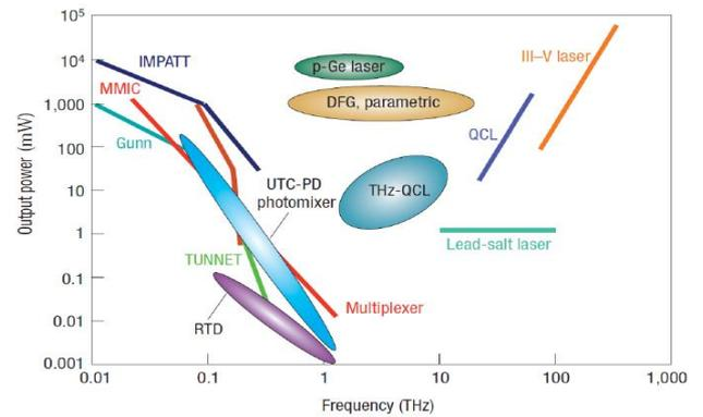
Figure 2: Reported THz-emission power output as a function of frequency: the terahertz-gap, the lack of strong and reliable THz sources, is evident in sub millimeter-wave range. (15)
