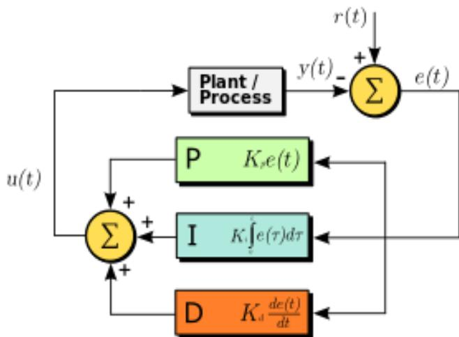
Figure 2. Block diagram of a PID controller in a feedback loop
