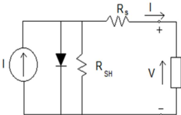
**Figure 1. Single diode model of a PV cell**
