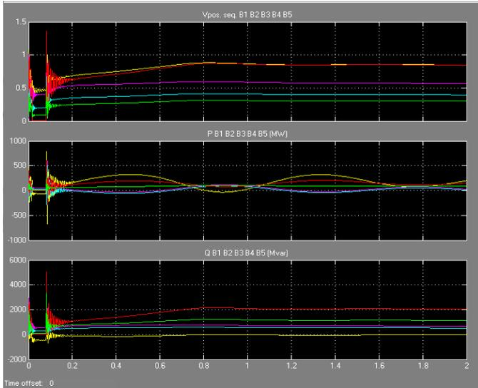
**Figure 1.4** Scope outputs of voltage, active power and reactive power measurement
