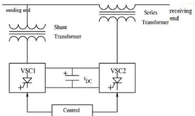
Figure 1.1 Block diagram of UPFC
